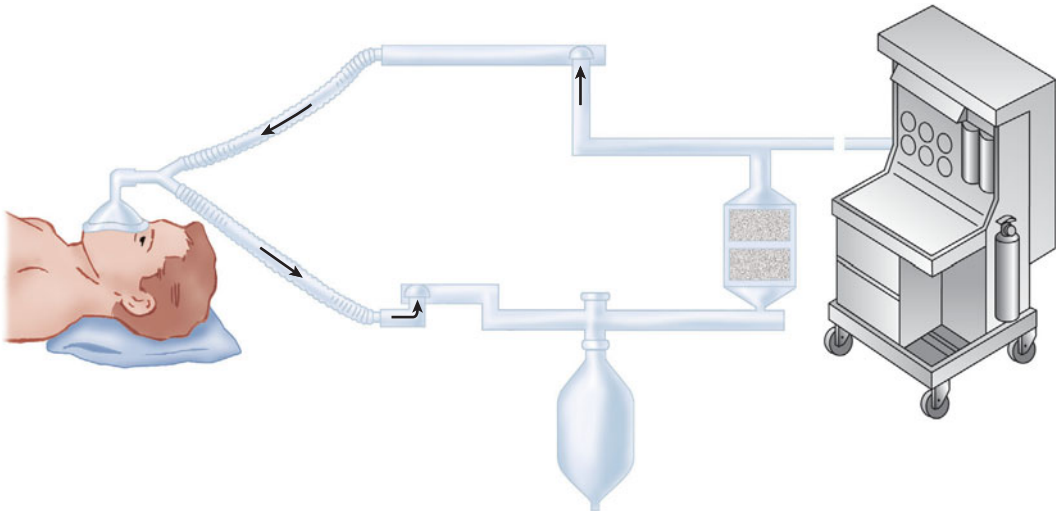
FIGURE 3-1 The relationship between the patient, the breathing system, and the anesthesia machine.
